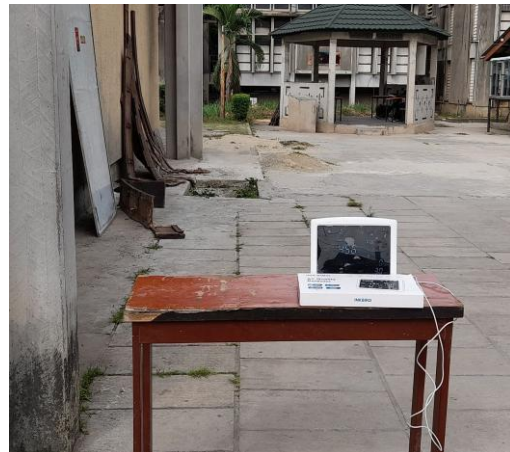
(b) Inkbird air quality monitor for outdoor air recording
