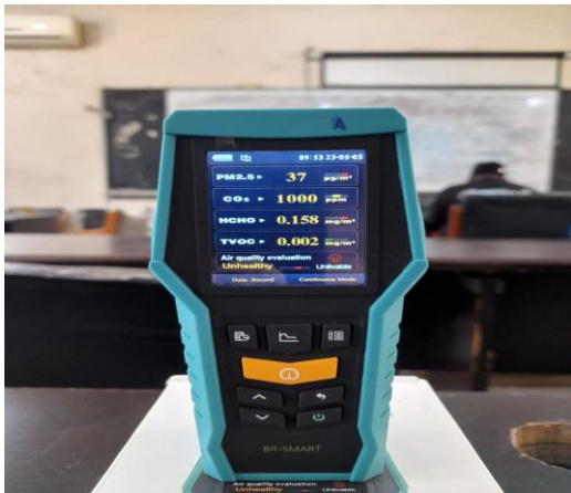
(a) Portable Hand-held Br-smart air quality monitor, for indoor air recording
